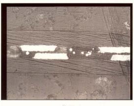
The photos show cross-sections of bonded connections with the ELATECH 2-component epoxy, filled with Ni spheres of 7-9 µm size.
