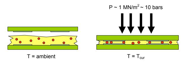
A vertically conductive connection is formed by compressing and curing an epoxy glue, which is filled with metal spheres (or metallized plastic spheres), between two flexible printed circuit boards with matched contact pads. The applied pressure reduces the thickness of the glue layer down to the diameter of the spheres. The concentration of spheres in the glue is chosen such, that contacts between spheres are rare; in particular the probability of contacts between adjacent pads is negligible.
